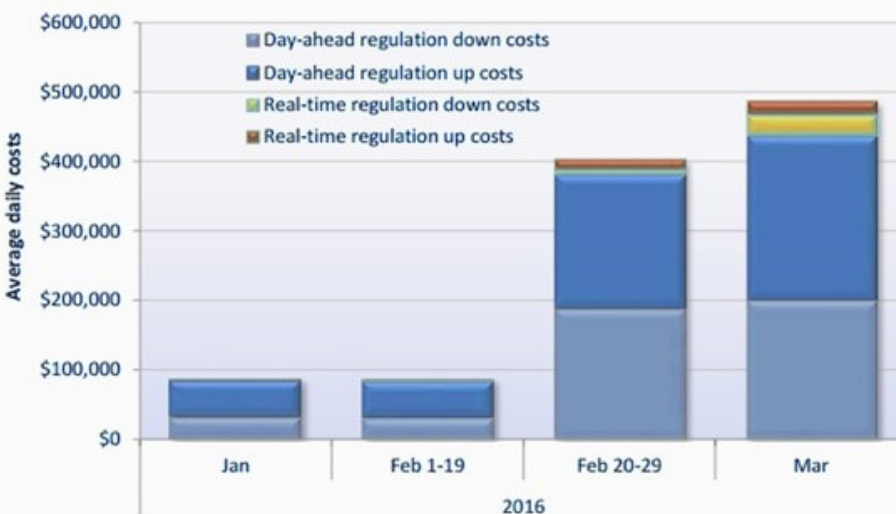
Average daily regulation procurement costs increased sharply after CAISO increased regulation requirements in late February. Source: CAISO
